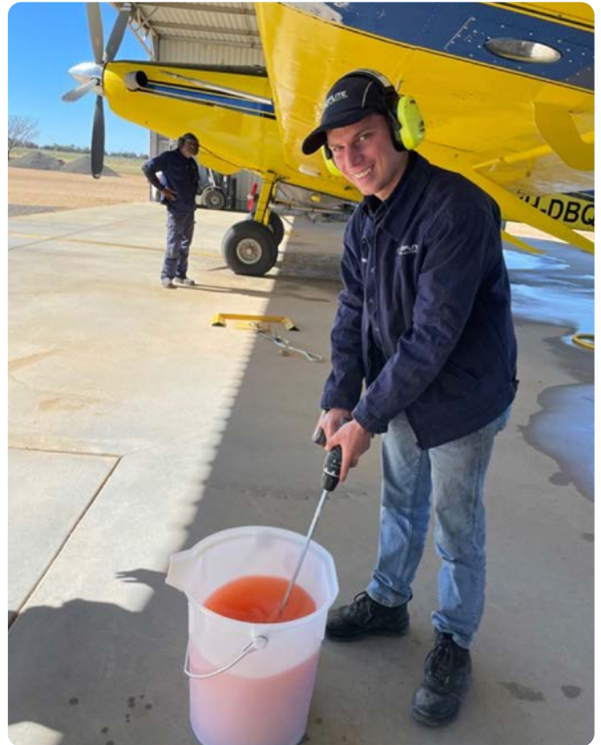
Figure 13 – A small batch of Magnet blank mixed with red dye being mixed to calibrate for droplet size.
