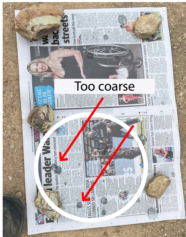
Figure 12 – Droplet size is too coarse
