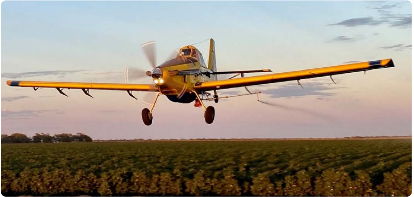
Figure 1 – AT802 applying Magnet to a cotton crop *note the low rate and single Bickley boom.
