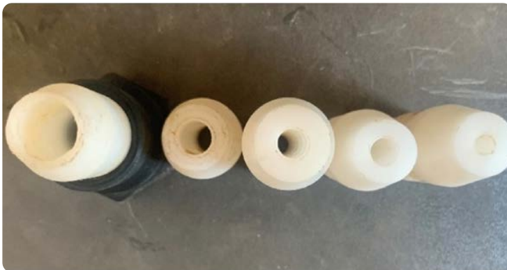
Figure 7– Nozzle tips made from nylon block can screw into check valve for easy changeover
