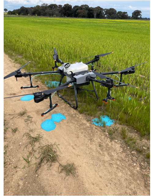
Figure 10 – A drone calibration using the Magnet blank recipe
